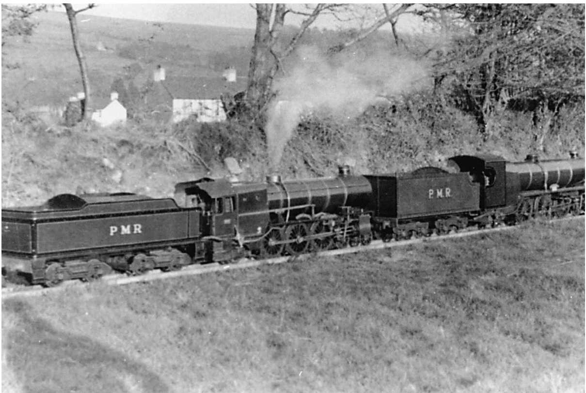
Kelly Bray 1948. Here we see George Dingle's 10¼" gauge railway at Kelly Bray, in a field adjacent to his yard, with his two 4-6-2s. Left is the Bullock and right the Thurston. These two photographs can be dated to 1948 - the Bullock locomotive has a raised running plate over the cylinders, altered when George Woodcock rebuilt the locomotive during winter 1947/1948. The Thurston locomotive was sold on over the winter of 1948/1949. Both locomotives have "PMR" on their tenders - presumably denoting Plymouth Miniature Railway, or Paignton Miniature Railway for the Bullock. The latter is clearly in steam.
